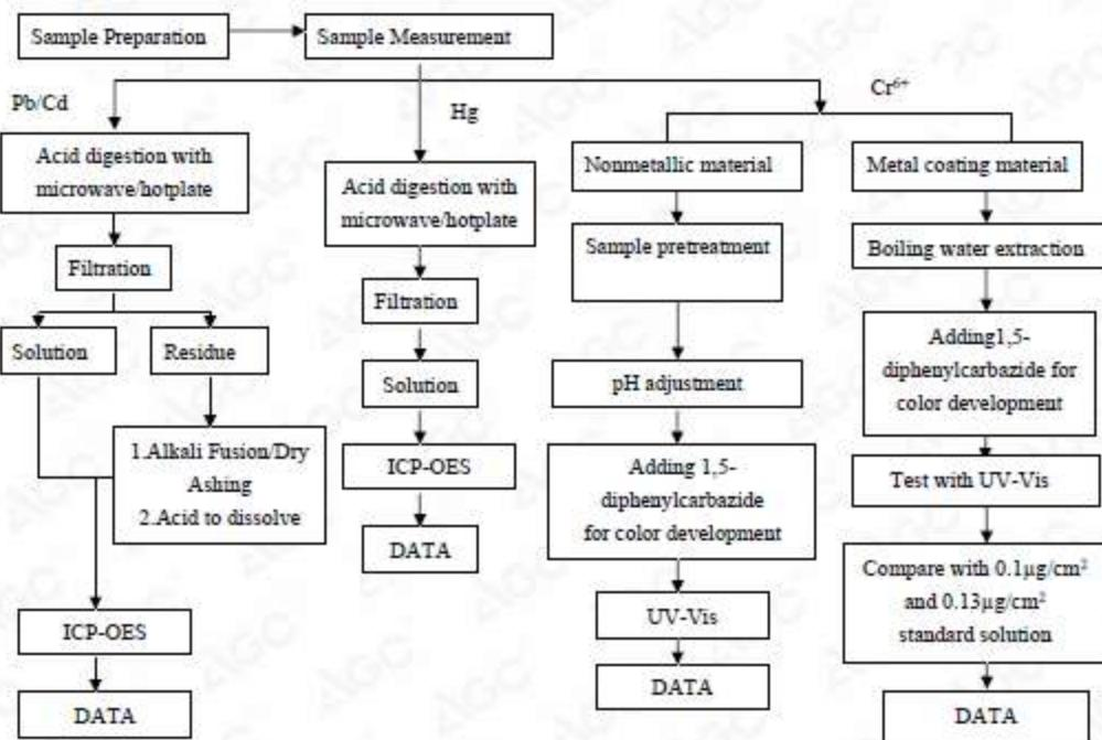
These samples were dissolved totally by pre-conditioning method according to above flow chart (Cr<sup>6+</sup> test method excluded)
