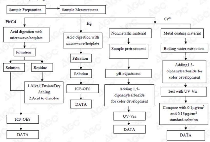
These sample were dissolved totally by pre-conditioning method according to above flow chart (Cr6+ test method excluded)
